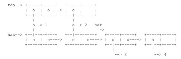
Note how 'foo' and the first half of 'baz' use the \*same\* objects for their elements -- copying a list only copies its cons cells, its elements are reused. Also note how the variable 'bar' actually references the mid-point of 'baz' since the last list in an 'append' call is not copied.
